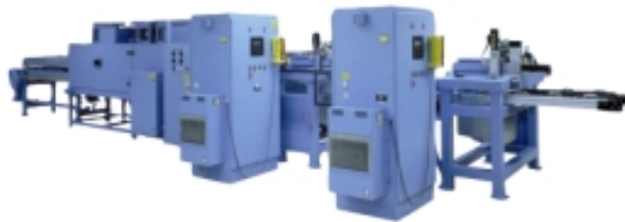
Figure 5. A turnkey system for dispensing and curing FIPG. A high quality flexible automated system will be fully programmable in three axes.
