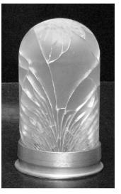
Broken globe held in place by silicone coating.
