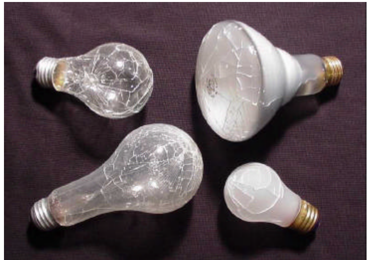
Broken light bulbs held in place by silicone coating.
